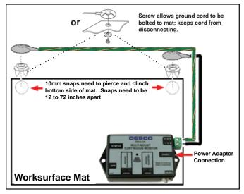
Figure 3. Installation method #1 of the Multi-Mount Continuous Monitor
