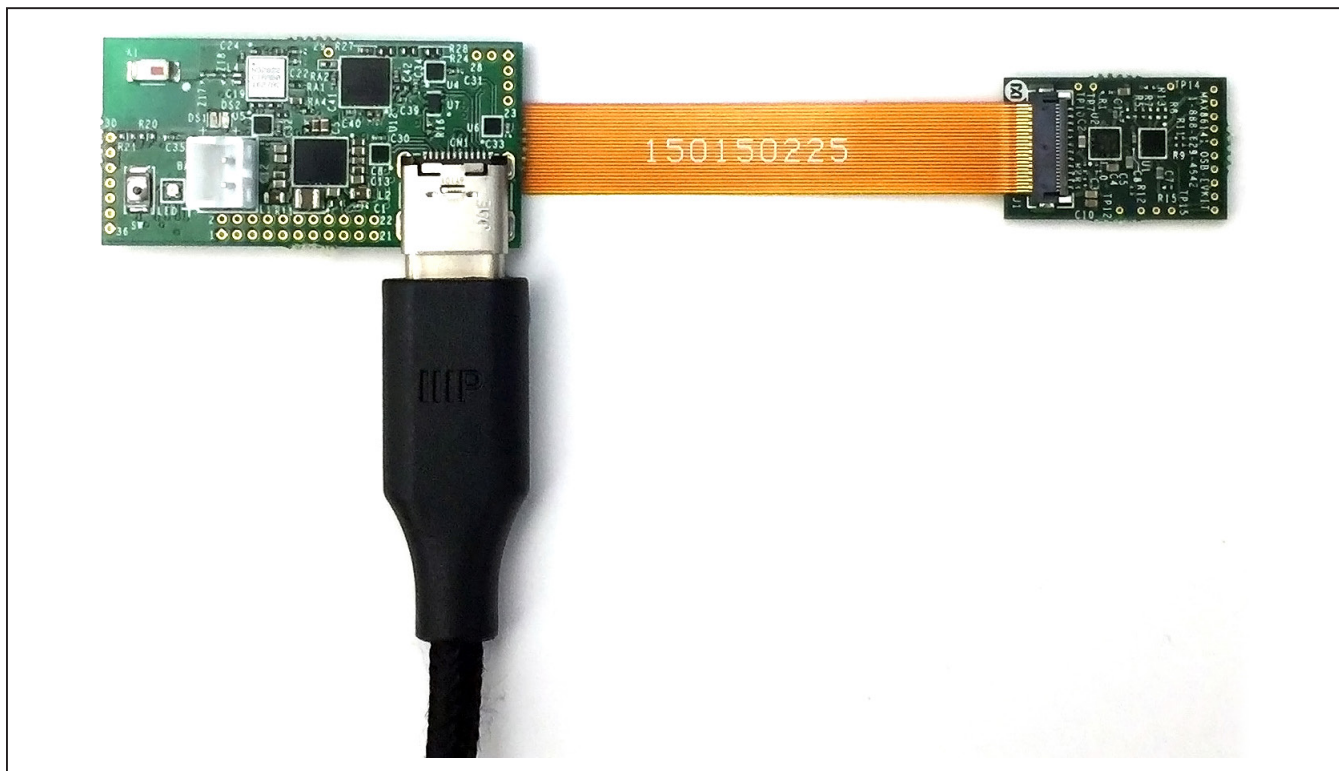
Figure 11. Hardware Setup (MAX86141 EVSYS Micro PCB)
