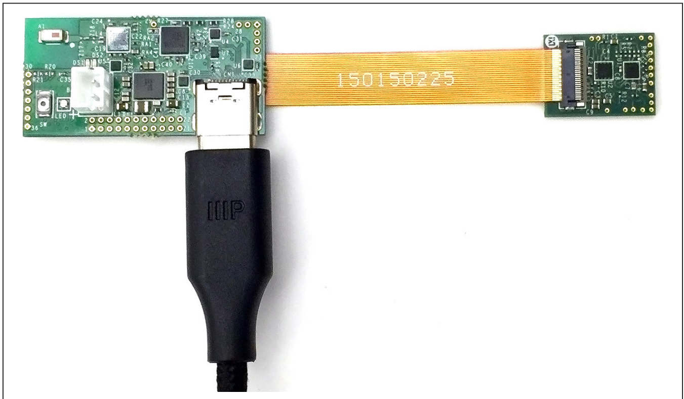
Figure 9. Hardware Setup (MAX86140 EVSYS Micro-PCB)
